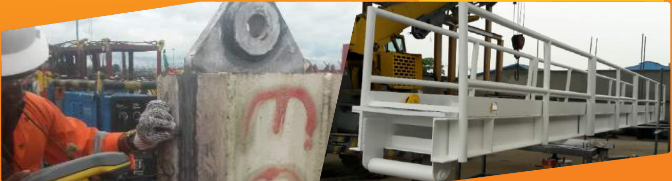
Ultrasonic Testing of ROV Basket Padeye for Egina
