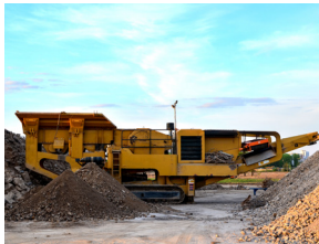
Rock Quarry Equipment (Jaw Crushers)
